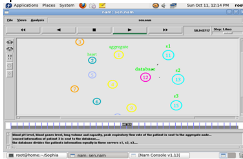
Figure.5. Node 2 senses heart of patient 1 and sends data to the aggregate node
